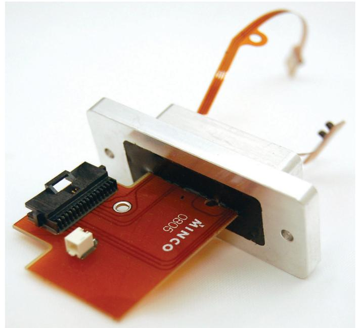
Creative use of materials can solve many feedthrough challenges, such as this hybrid rigid/flex circuit board feedthrough.
